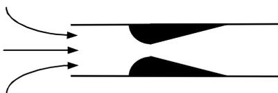
$$\left. \begin{matrix} P_0 \\ T_0 \\ H_0 \end{matrix} \right\} \rho_0 \quad \begin{matrix} Q_0 \text{ (g/s)} \\ Q_{V0} = \frac{Q_0}{\rho_0} \text{ (l/s)} \end{matrix} \quad \Rightarrow \quad \left. \begin{matrix} P_1 \\ T_1 \\ H_1 \end{matrix} \right\} \rho_1 \quad \begin{matrix} Q_1 \text{ (g/s)} \\ Q_{V1} = \frac{Q_1}{\rho_1} \text{ (l/s)} \end{matrix}$$
